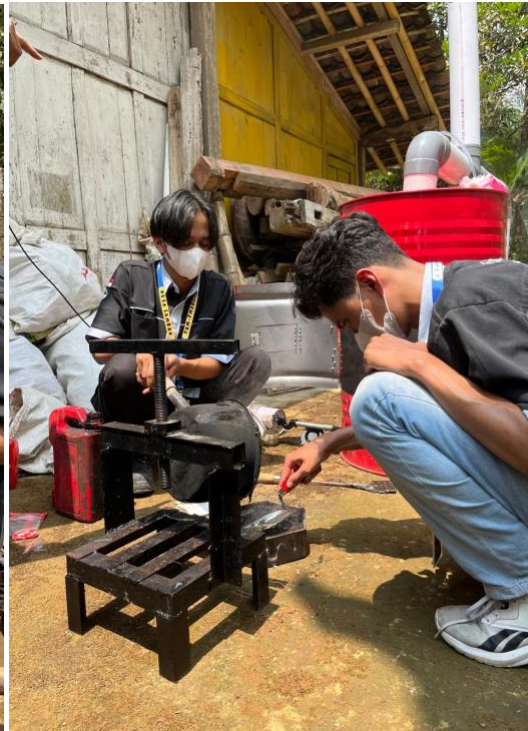
Figure 9. Process of pouring a mixture of plastic waste, cement and sand into the mold
