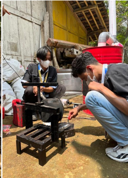
Figure 9. Process of pouring a mixture of plastic waste, cement and sand into the mold
