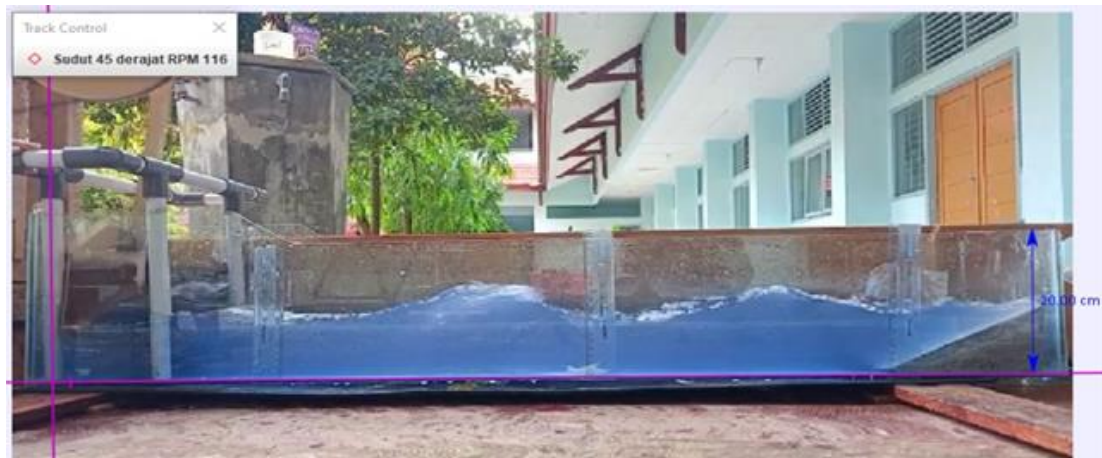
FIGURE 6. The wave in laboratory scale of wave simulator with wedge angle of 45^\circ
