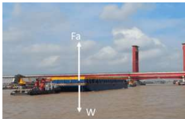
FIGURE 2. Buoyancy and weight on barges
