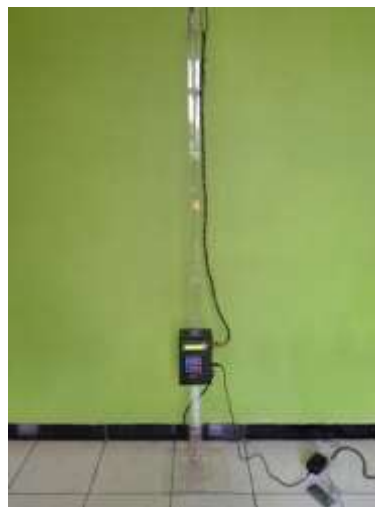
FIGURE 3. Arduino UNO-based viscosity determination tool circuit
