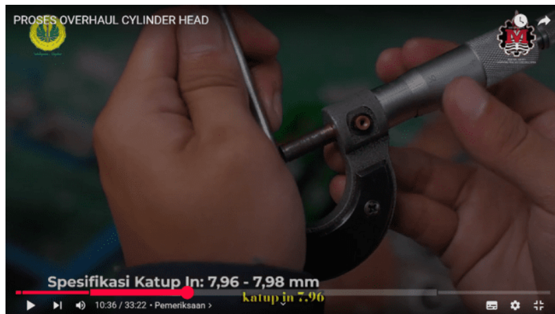
Gambar 4. Video Proses Overhaul Cylinder Head
