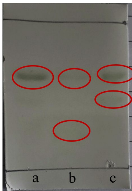
Figure 7. TLC analysis of pheophytin (a), Nd–pheophytin (method 1) (b), and Nd–pheophytin (method 2) (c).
