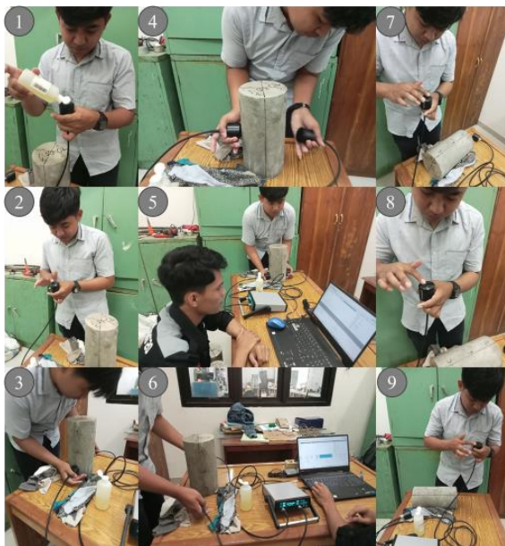
Gambar 6. Pengujian Ultrasonic Pulse Velocity (UPV)
