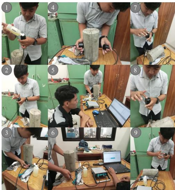
Gambar 6. Pengujian Ultrasonic Pulse Velocity (UPV)
