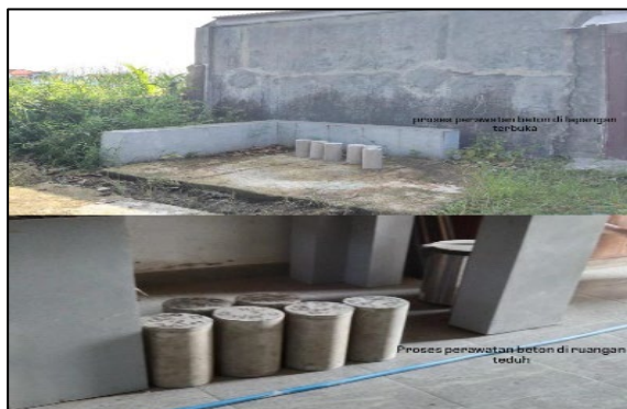
Gambar 1. Proses Perawatan Beton
