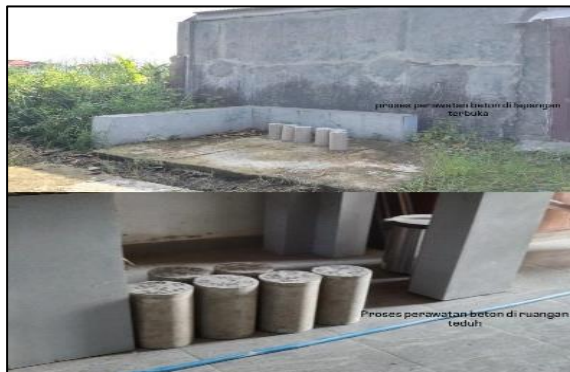
Gambar 1. Proses Perawatan Beton
