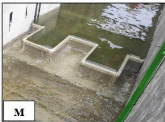
Gambar 3. Bendung Labirin Tipe Rectangular (Folded) (Tanga dkk., 2023) .
