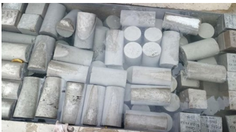
Gambar 6. Proses Perawatan Beton
