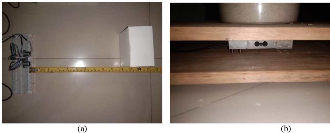
GAMBAR 1. (a) proses karakterisasi sensor HY-SRF05 dan (b) proses karakterisasi sensor load cell single-point
