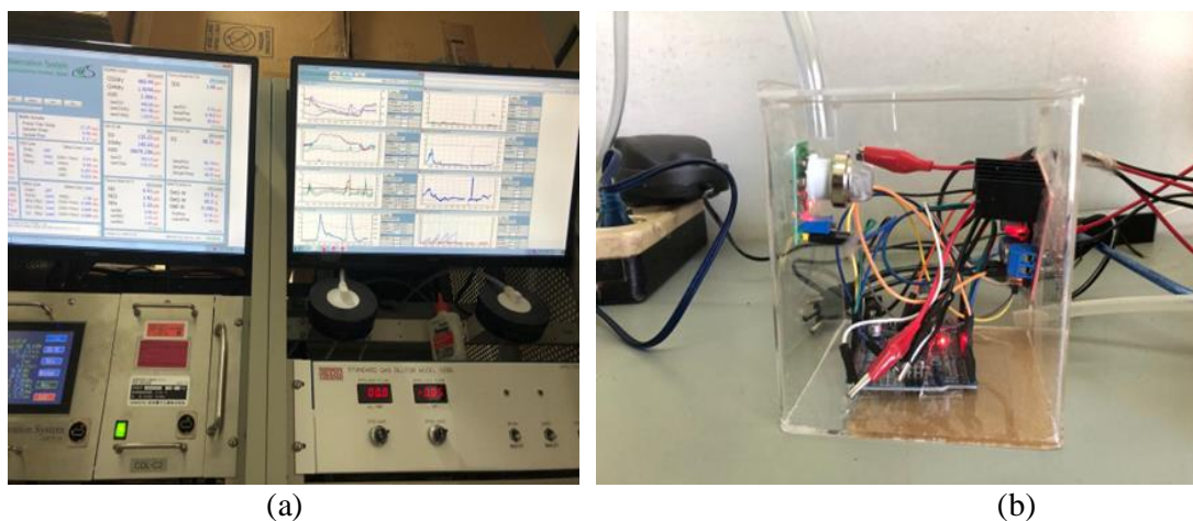
GAMBAR 2. (a) Gas analyzer G2203 and G2301 Picarro; (b) Proses Karakterisasi Sensor Gas
