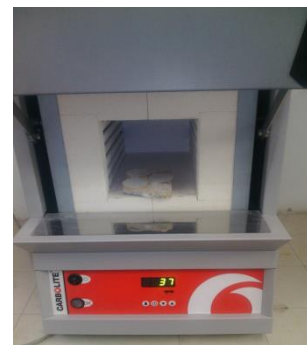
Gambar 1. Proses Sintering didalam furnace
