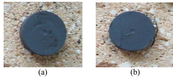
Gambar 1. Material hasil sintering (a) material \text{BaCoTiFe}_{16}\text{O}_{27} dan (b) \text{BaCoTiFe}_{15.8}\text{Co}_{0.1}\text{Ti}_{0.1}\text{O}_{27}
