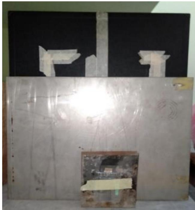
**Figure 1.** Layer placement during irradiation
