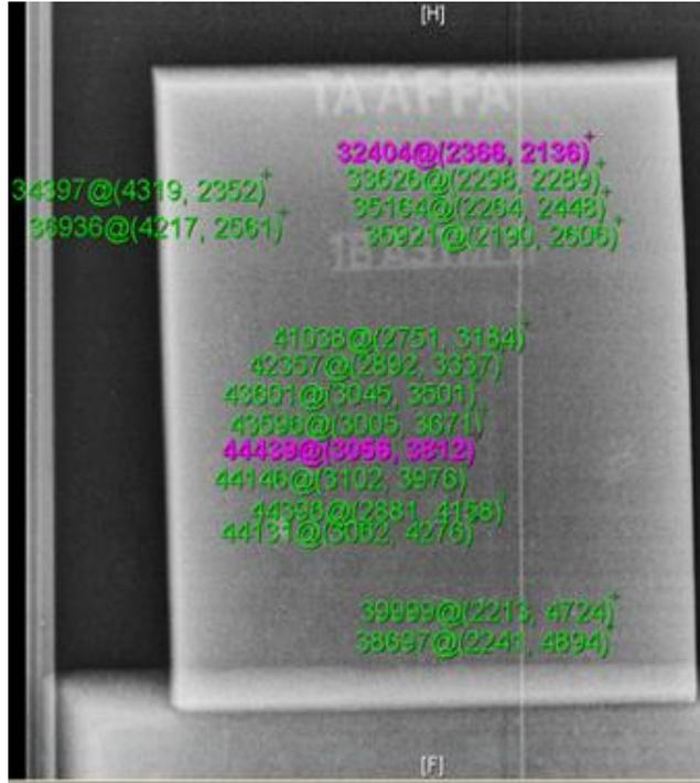
**Figure 4.** Radiographic image without filter layer, with energy 5 MeV
