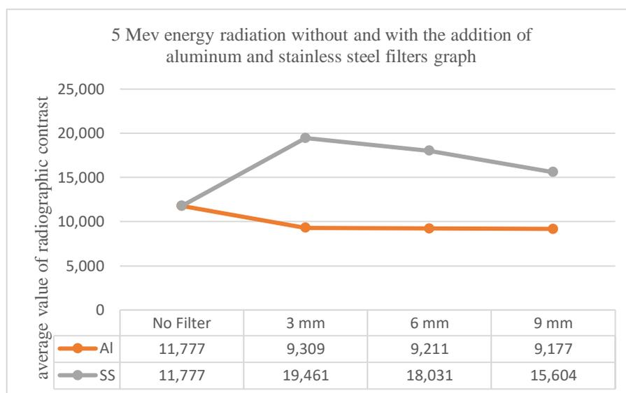
**Figure 3.** Graph of 5 MeV energy irradiation without and using aluminum and stainless steel filter
