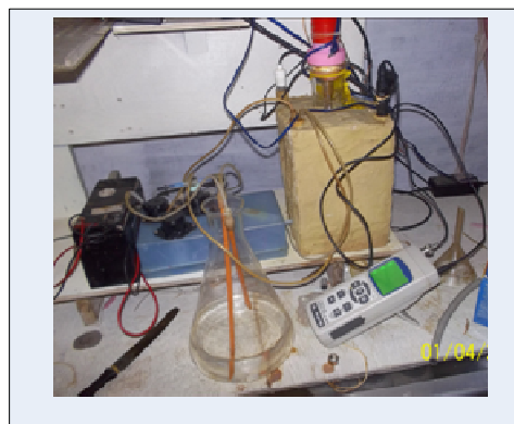
Figure 1. The picture of the flow injection synthesis of CuZnFerrite co-precipitation reactor with datalogger of pH and temperature acquisitions \
