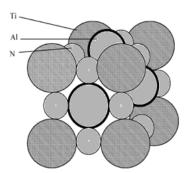
**Figure 1** TiAlN structure (fcc-NaCl structure) models schematic. Ti occupies fcc positions and the cube corners. Al occupies the octahedral sites at the centers of the cube edges [16].
