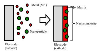
Figure 3. Electrodeposition of nanocomposite
