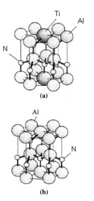
**Figure 2** Model schematic of (a) hexagonal-TiAlN; (b) hexagonal-AlN [17].
