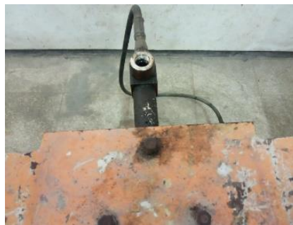
Gambar 4 Pipa Drat CTM (Compression Testing Machines)
