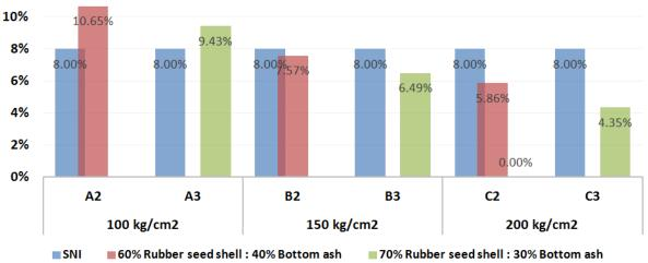
FIGURE 1. The water content of rubber seed shell and coal bottom ash briquettes.
