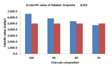
FIGURE 6. The calorific value of Halaban wood charcoal and coal bottom ash briquettes.
