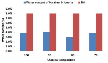
FIGURE 2. The water content of Halaban wood charcoal and coal bottom ash briquettes.
