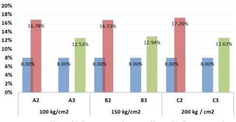
SNI 60% Rubber seed shell: 40% Bottom ash 70% Rubber seed shell: 30% Bottom ash FIGURE 3. The ash content of rubber seed shell and coal bottom ash briquettes.
