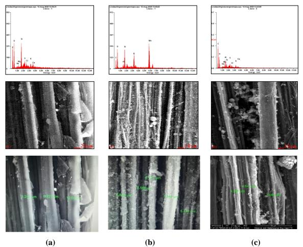
FIGURE 1. The SEM-EDX results of purun tikus: (a) without treatment, (b) KMnO<sub>4</sub> 2% treatment, (c) NAOH 5 % treatment.
