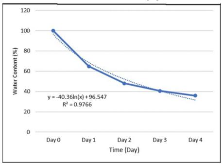
**FIGURE 2.** Graph of data 2 Correlation of Time (days) and Water Content of Dried Fish (%) For Mass 863 grams.
