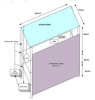
FIGURE 1. The fish drying Using a Solar Panel-Based Dryer system
