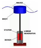
FIGURE 4. Permanent magnet linear buoy system
