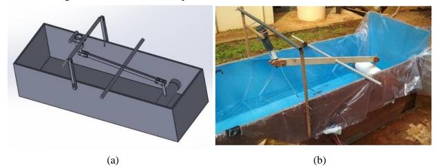
FIGURE 13. (a) Overall design (b) Original look of linear generator system with vertical configuration
