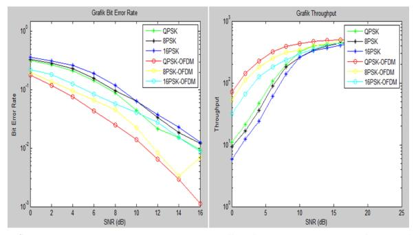
FIGURE 7. BER vs SNR and Throughput graph on the effect of OFDM usage on system performance with QPSK, 8PSK and 16PSK
