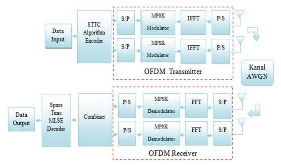
FIGURE 5. Block Diagram of STTC
