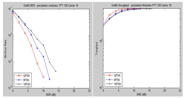
**FIGURE 10**. Graph of BER vs. SNR and throughput on the effect of changes in modulation on system performance with FFT128 and carrier 16
