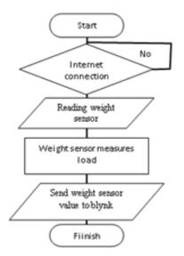
FIGURE 5. Weight sensor monitoring test flowchart
