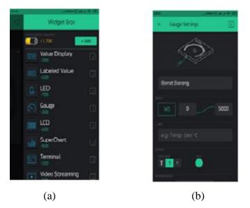
**FIGURE 3**. the maker of the monitoring system for the existence of goods in the box with the blynk application, (a) adding a gauge widget, (b) setting the gauge widget.
