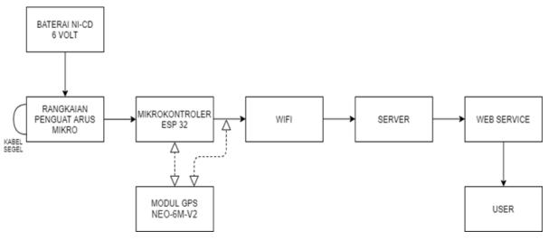
FIGURE 1. Smart Seal Block Diagram
