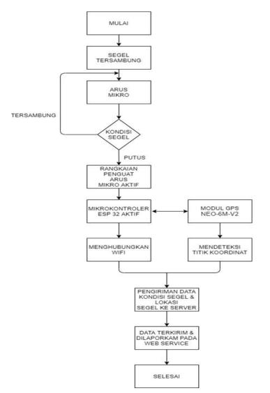
FIGURE 2. Smart Seal Principle Diagram
