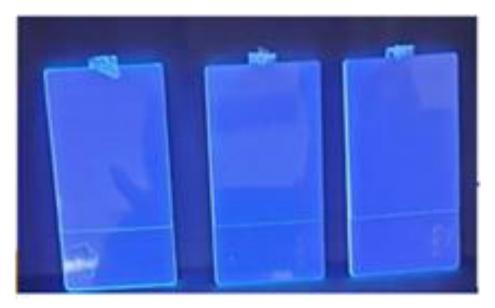
FIGURE 4. Thin plates from extrusion process irradiated by UV light
