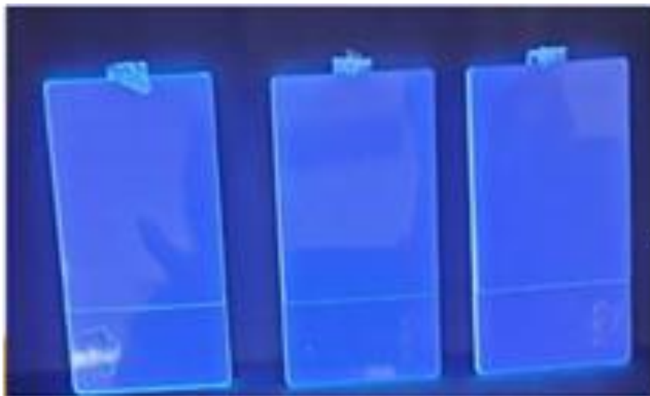
FIGURE 4. Thin plates from extrusion process irradiated by UV light
