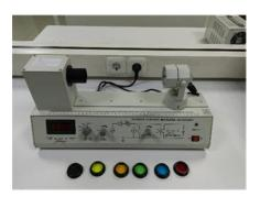
FIGURE 1. Photoelectric Effect Experiment Set
