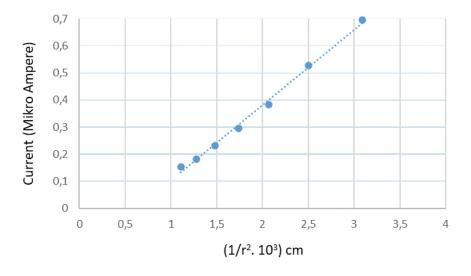
FIGURE 5. The correlation between the distance of the light source and the resulting current
