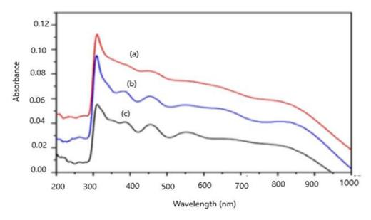
**FIGURE 4.** Spectrum of the  $0.3BaTiO_3 - 0.7BaZr_{0.5}Ti_{0.5}O_3$  thin film with (a) at 700°C, (b) at 750°C and (c) at 800°C
