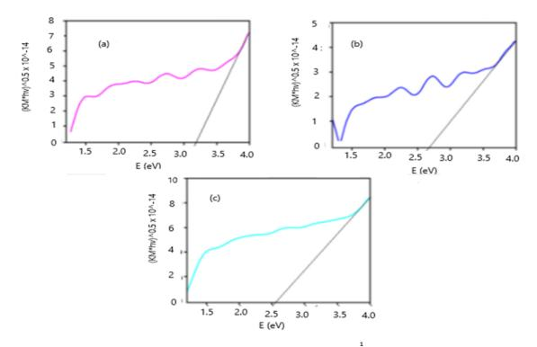
**FIGURE 5.** Determination of Eg Value from the relationship  $(F(R) hv)^{\frac{1}{2}}$  and hv Energy (eV), (a) at 700°C, (b) at 750°C and (c) at 800°C
