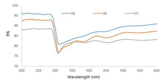
**FIGURE 3.** UV-Vis reflectance curve of  $0.3BaTiO_3 - 0.7BaZr_{0.5}Ti_{0.5}O_3$  thin film annealed at (a) 700°C, (b) 750°C and (c) 800°C.
