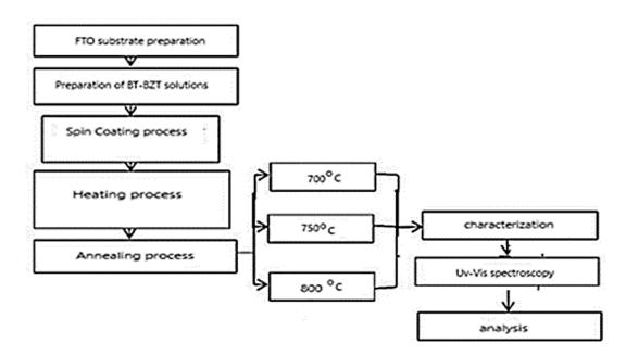
FIGURE 2 : Flow chart making of thin film BT-BZT.
