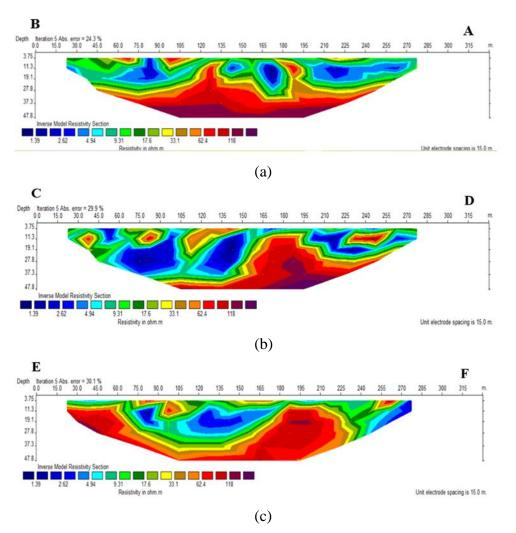
FIGURE 5. The 2D resistivity profiles (a) line 1, (b) line 2, and (c) line 3
