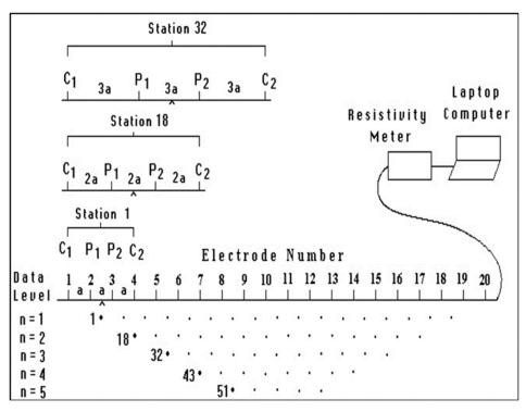
**FIGURE 2.** The 2D resistivity measurement scheme of the Wenner array with "a" as the electrode interval and "dot" point as the datum representation [24]
