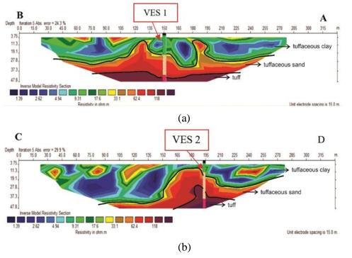
FIGURE 6. The correlation of 1D results and 2D resistivity profiles (a) VES 1-line one and (b) VES 2-line two
