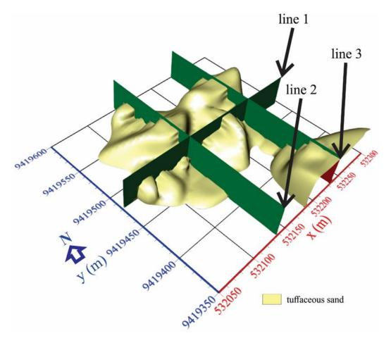
FIGURE 8. The 3D modeling of the groundwater layer
