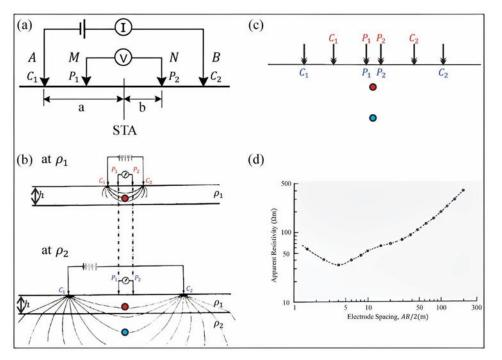
**FIGURE 1.** The 1D measurement (a) array setting, (b) the electrodes are shifted to the right and left from the central point (STA), (c) depth estimation of the datum point from each shifted electrode, and (d) the datum reconstruction on a chart between resistivity value and half distance "a" or AB/2 (modified from [10])
