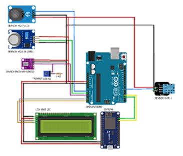
FIGURE 1. Circuit of Gas Sensor
