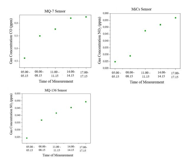
FIGURE 5. Gas concentration measurement in environment in different time interval.
