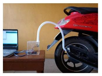
FIGURE 3. Vehicle's exhaust gas sensing measurment setup.
