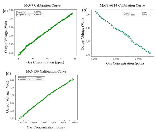
FIGURE 2. Calibration curve for each gas sensor: (a) MQ-7, (b) MiCS-6814, (c) MiCS-136.
