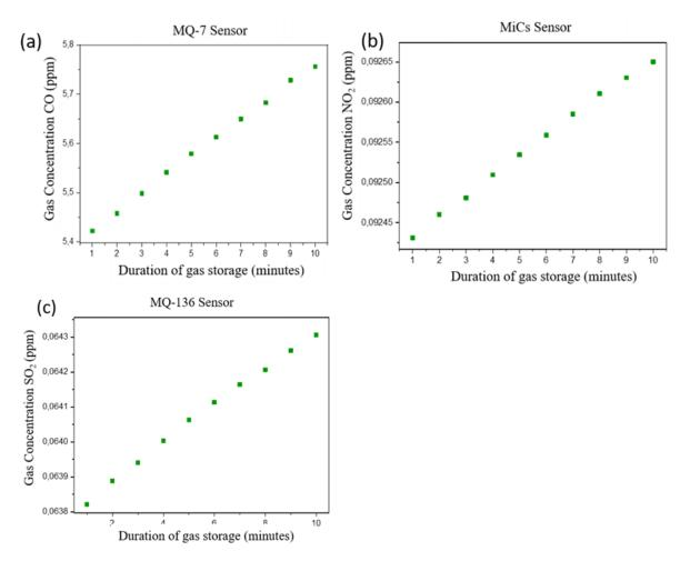
FIGURE 4. Gas sensor measurement on vehicle's exhaust with different gas storage duration for each sensor.
