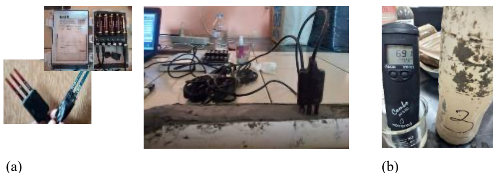
FIGURE 4. (a) Mud samples measured ex-situ with Decagon EM-50; (b) Water samples measured ex-situ with Hanna Combometer.
