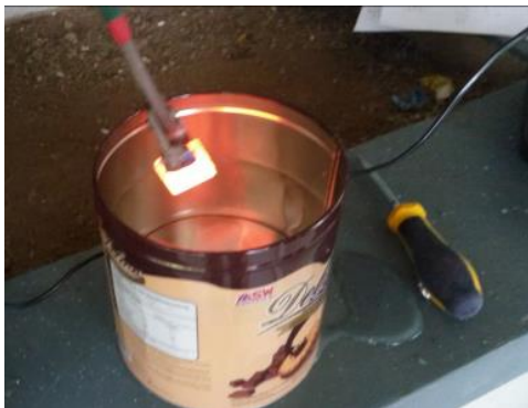
FIGURE 6. Quenching process of heated sample.
